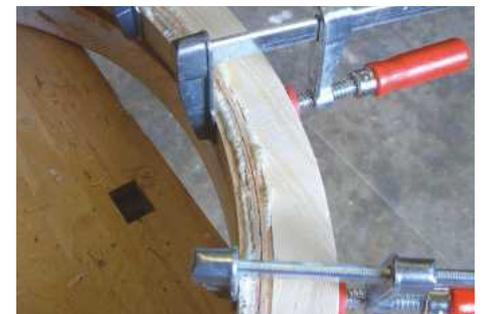
▲ Pic.12 Glazing strips are laminated from 2mm thick oak strips, glued together inside the frame
